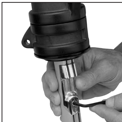
Loosen screw one revolution only .
