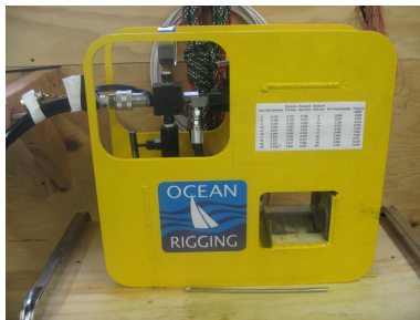
Ocean Rigging's Rod Cold Head Machine, Fabricating rod rigging, in house
